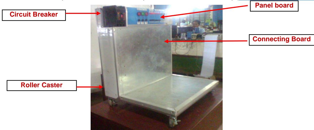
Figure 7: The Tabletop Industrial Motor Control Trainer
