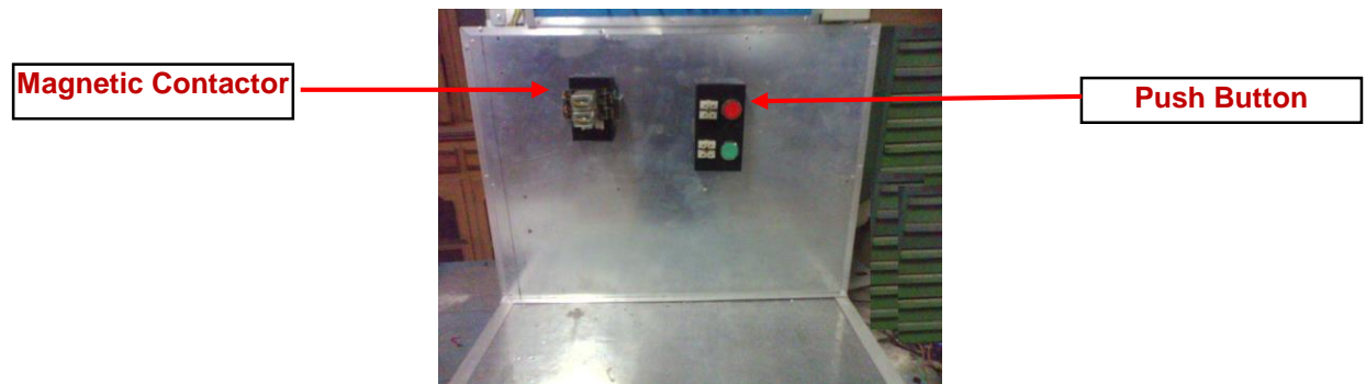
Figure 8: The Metallic Wiring Board of the Trainer
