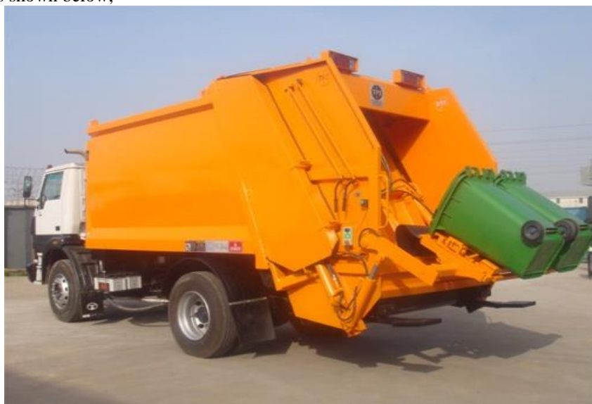
Figure 1: A Compression lifting Refuse from a residential Apartment.
