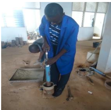
Compacting soil with rammer
