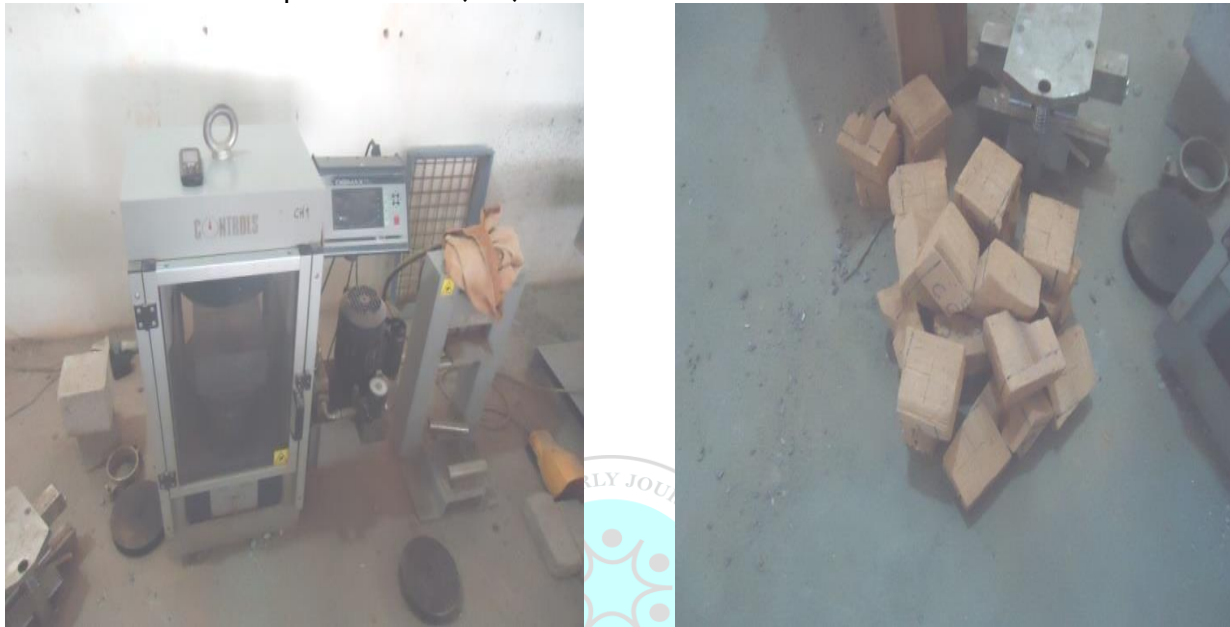
Figure 3.10 Testing the Flexural Strength of Bricks by means of three – point Bending Moment.
