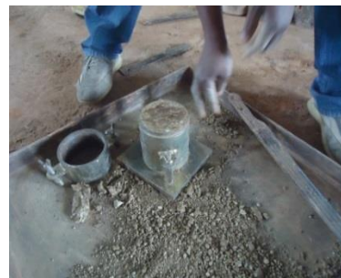
leveled soil according to mould
