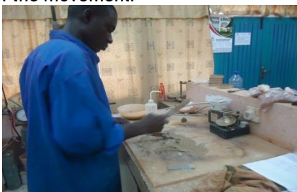
Preparing samples for all Atterberg tests
