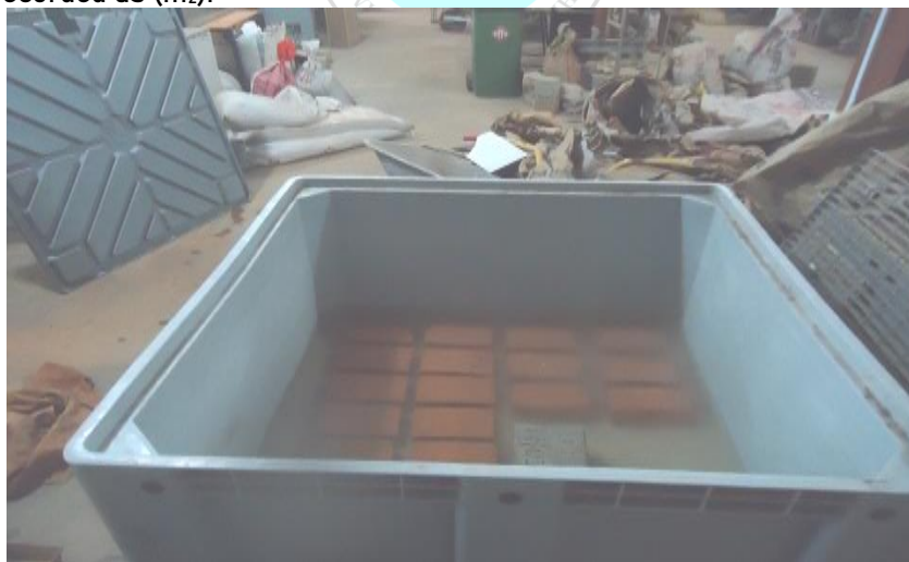
Figure 3.8 Bricks Completely Immersed in water trough for 24 hours for Water Absorption Water absorption, percentage by mass, after 24 hours emersion in cold water is given by the formula.
