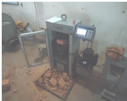
Figure 3.7 Testing Compressive Strength of Bricks and automatic graph plotted during the test
