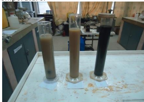
Samples in 1000ml cylinder for hydrometer analysis
