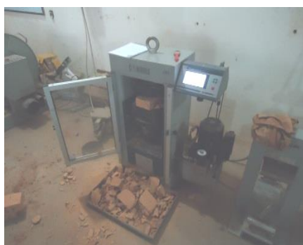
Figure 3.7 Testing Compressive Strength of Bricks and automatic graph plotted during the test
