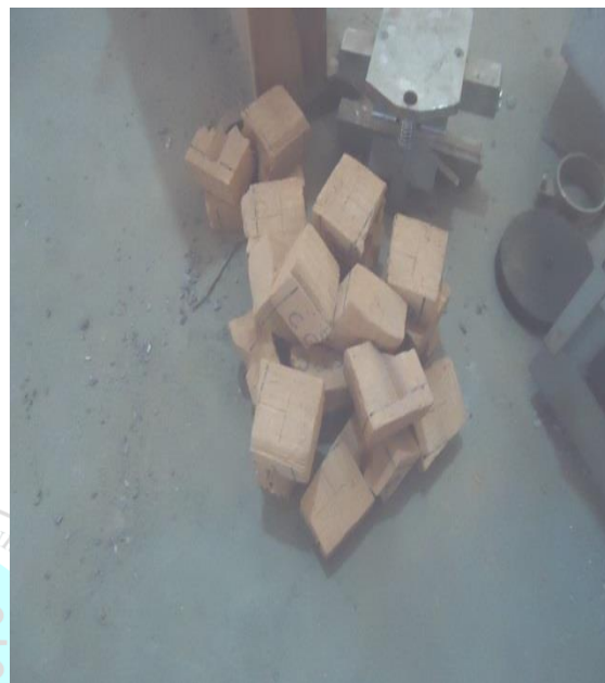
Figure 3.10 Testing the Flexural Strength of Bricks by means of three – point Bending Moment.
