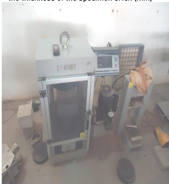
Figure 3.10 Testing the Flexural Strength of Bricks by means of three – point Bending Moment.
