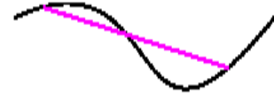
A function that is neither concave nor convex. The line segment shown lies above the graph at some points and below it at other points.
